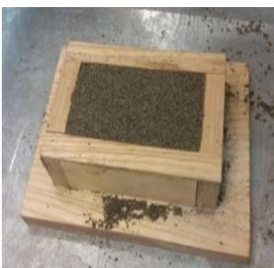
Figure 2: Casting of the brick
