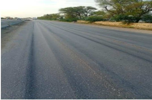
Fig: 4 Excessive rutting in newly laid HMA having 1 Layer of AWC (5cm) Class B & 2 layers of ABC (16cm) Class B N-55
