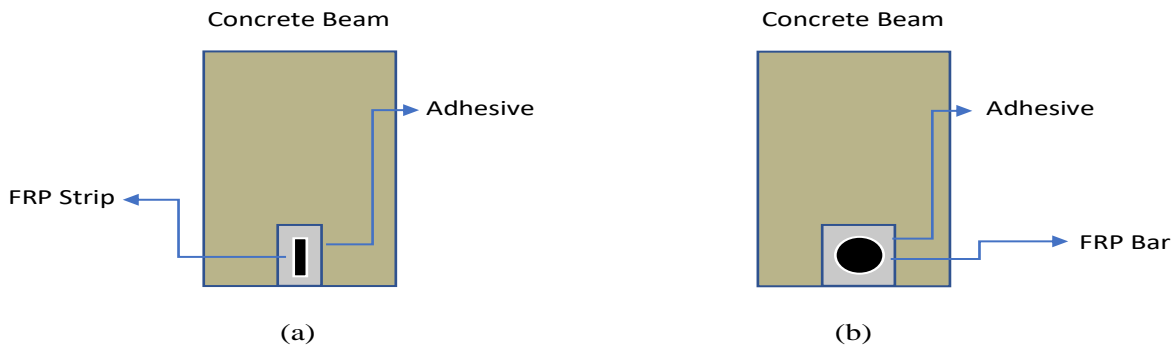
Figure 1 Cross-section of NSM-FRP
