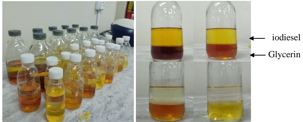
Figure 3: Product samples (a), biodiesel and byproduct glycerin from transesterification (b)
