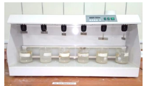
Figure 2: Jar Test Apparatus
