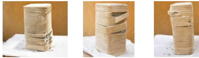
Figure 3. Failure modes of specimens; (a) S R21 L1; (b) R1.5 R21 L1; (c) R2 R21 L2
