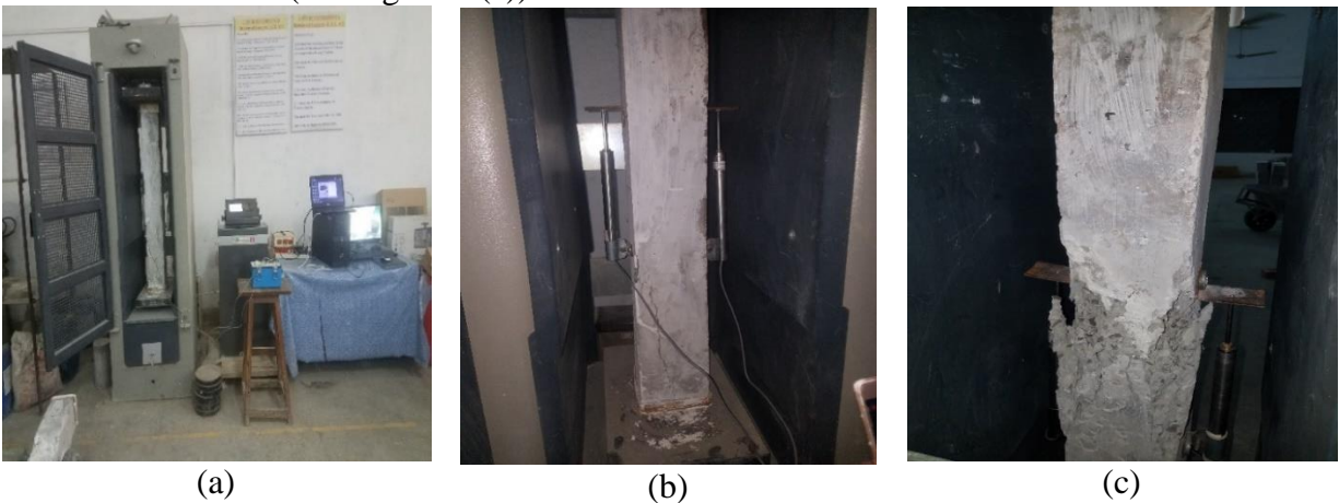
Figure 2: Compression testing of the columns (a) Test setup (b) Arrangement of LVDTs (c) Failed column after ultimate load
