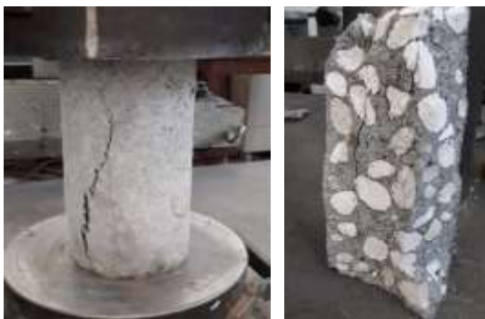
Fig. 5: Concrete Cylinder in compression test
