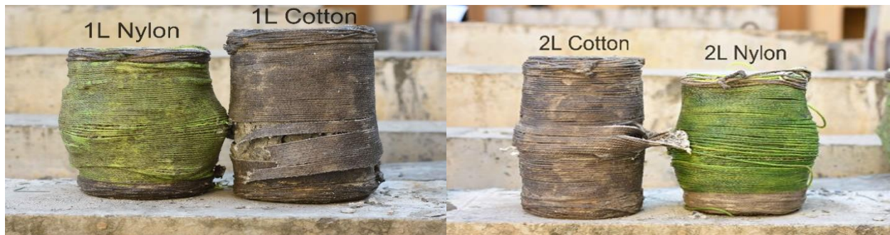
Figure 3: Typical failure mode of 1- & 2-layer NFRP confined specimens.
